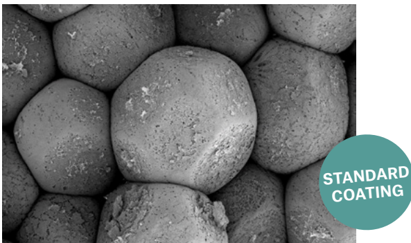
Figure 5: Fracture surface/broken cells example with customer standard coating . The surface is clean, which means that the block was separated at the fusion line between the beads, inducing a poor fusion.
